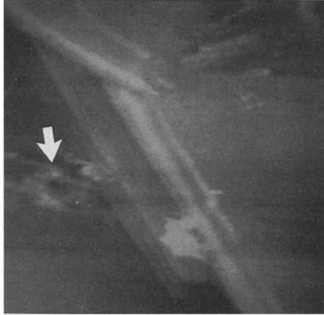
Fig. 3: STM image of a PB-1 film deposited onto HOPG. Imaging was done in air over an area of 250 \times 250 \text{ nm}^2 , I_t = 0.6 \text{ nA} , V_t = 463 \text{ mV} , tip positive. The extended flakes consist of polymeric material. Note the fibrillar structure of the film at the edge of the flake.
